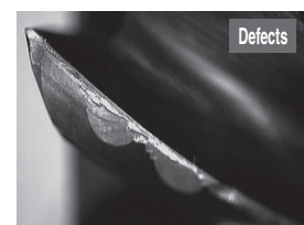
After machining 10 min
