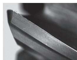
After machining 50 min
