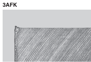
Burr Comparison after Machining (Internal evaluation)
