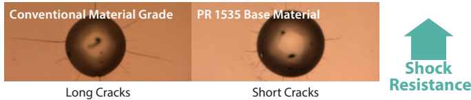
Cracking Comparison by Diamond Indenter (Internal evaluation)
