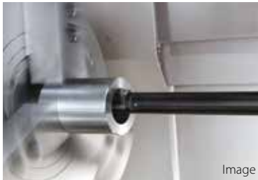
KAV-G20-10D / KAVH20-SCLCR09 CCMT09T304PP Overhang length: 140 mm (7D) / 200 mm (10D) Workpiece material: SCM435
