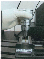
(Figure 7) Torsional strength test of abutment screw (n=5)
